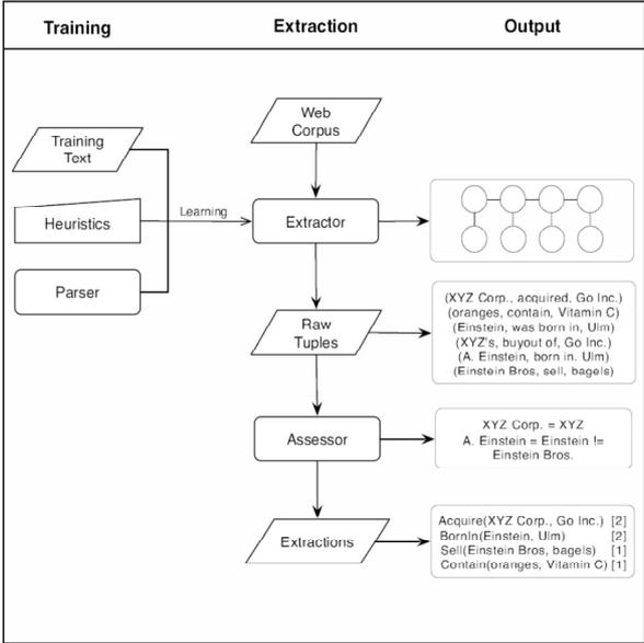
Figure 5. TextRunner architecture <sup>38</sup>
