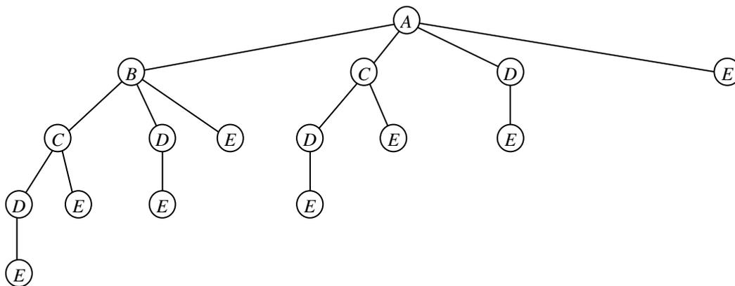
**Figure 18. Worst case scenario tree construction for step 4 merging function**
