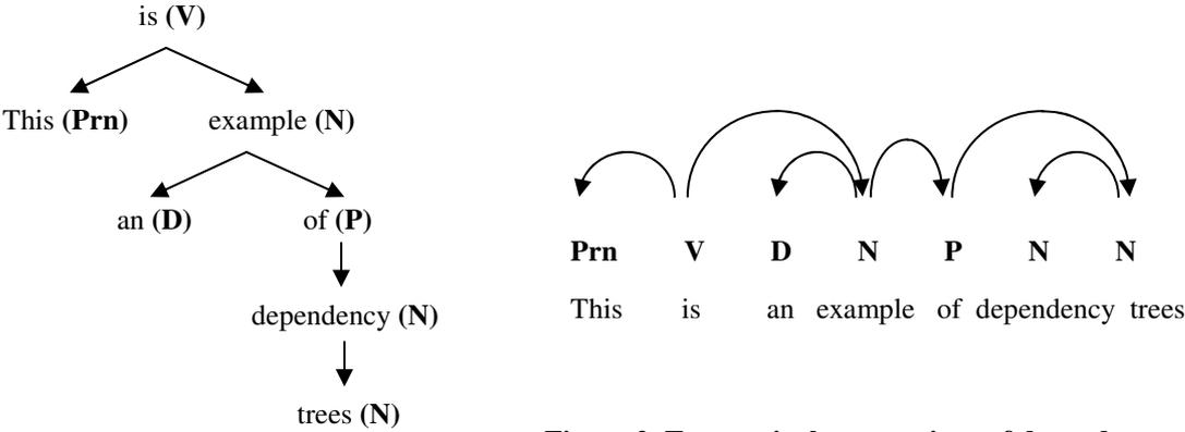
**Figure 2. Two equivalent notations of dependency trees**
